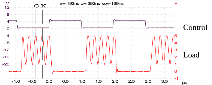
A sample of chopping of 50MHz, 4V signal
