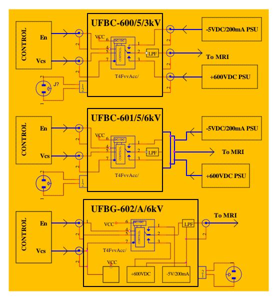
Ultra-fast, bipolar pulse generating devices deliver bias voltages for controlling conductivity of high-voltage PIN diode during real-time dynamic MRI scanning. Brief descriptions of each device, useful attachments, and prices are included.
