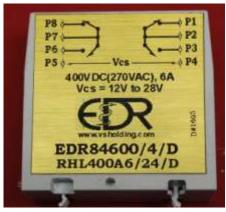
The DPDT physical size varies and mostly depends on output voltage/current rating. For example P/N EDR84600/4/D or RHL499A6/24/D (DPDT) rated at 400 VDC (270 VAC), Id rms = 6-Amps, Id max = 40-Amps and Id pulse = 140-Amps is capable of driving almost 5 kW load (no external heat sink is required). Relays were encapsulated in a DIN box of 11"W x 11"H x 11" W. Larger packages are used for switching higher power.
